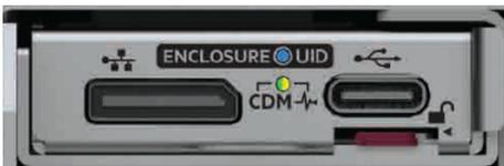
**Figure 1.** CDM on the back of an HPE Alletra Storage MP controller node. The Bluetooth dongle can be connected to the USB-C port
