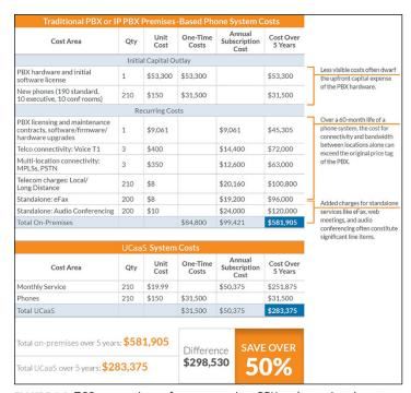
**FIGURE 2-3:** TCO comparison of an on-premises PBX and associated costs, and UCaaS.
