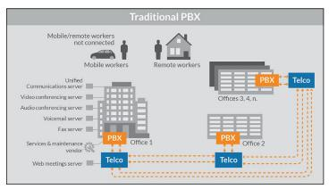
**FIGURE 1-1:** TDM PBXs provide limited integration with other apps and systems, and little or no support for mobile/remote workers.
